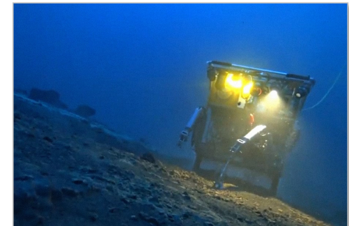
ROV Liropus 2000: An underwater robot capable of reaching depths of up to 2000 meters.
